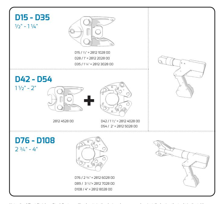
Note: the AIRnet Stainless Steel System will only attain the designed pressure when installed using the tools in the table above. Using other tools is not recommend, as this may lower the pressure rating.
