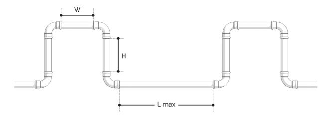
Long straight pipes will expand or contract due to temperature variations. To compensate for this effect, expansion loops or compensators are required. An expansion loop is a U-shaped construction that compensates the variation in length. Compensators are straight fittings specifically designed to allow axial movement. The number of expansion loops / compensators depends on the total length of the straight line and the maximum temperature variation.
